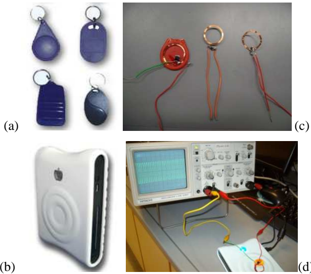
Figure 1.: Experimental materials: (a) represents four examples of Intergraded Circuit (IC) cards. (b) is an S8 IC card reader. (c) shows several disassembled IC cards with wires connected. (d) is an oscilloscope, which shows the signal from the IC card induced by the reader
